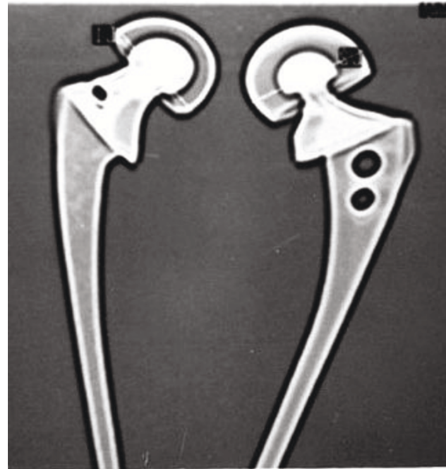
Figure 7 BHU bipolar prosthesis (right side) showing increased thickness of UHMWPE due to smaller diameter of the inner head.
